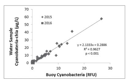
Cyanobacteria abundance detected by the buoy sensor was proportional to cyanobacteriachlorophyll *a* concentration collected and measured from a water sample.
