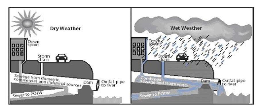
Volume of water in collector sewer during wet weather becomes 2.5 times more than volume of water in dry weather
