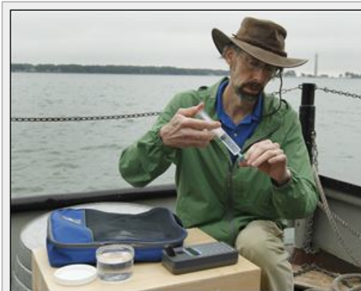
Dr. Rick Stumpf, of NOAA, demonstrates how to measure water samples with a fluorometer while on a boat in Lake Erie at Stone Laboratory on Put-in-Bay.
